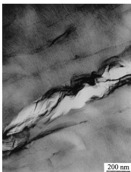
Fig. 3. Void formation between the folded silicate layers during the microtoming of the bulk nanocomposite.
